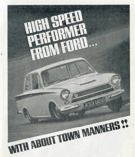
Cortina developed by Lotus. Twincam engine, 105 bhp at 5,500 rpm, Chapman suspension in the Lotus idiom. With Cortina's stamina and 5-seat comfort, trimmed for high-speed luxury. Close-ratio gears and a lower, lighter body. Full performance instrumentation. Special seats and a wood-rim wheel. Maximum speed 108 mph; 0 to 100 in under 30 seconds — with power brakes to match. From only £1,100 tax paid. Judge their performance for yourself
