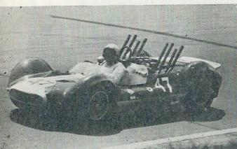
Bruce McLaren's 'rocket launcher'! This is the car which won last year's Guards Trophy race in the hands of Roger Penske, when it was called a Cooper Zerex Special. Since McLaren brought the car back to this country he has completely stripped and rebuilt it, and has fitted an Oldsmobile V8 engine. Now known simply as a Cooper-Oldsmobile, it won its first race in its latest guise - the Players 200, at Mosport Park, Canada.
